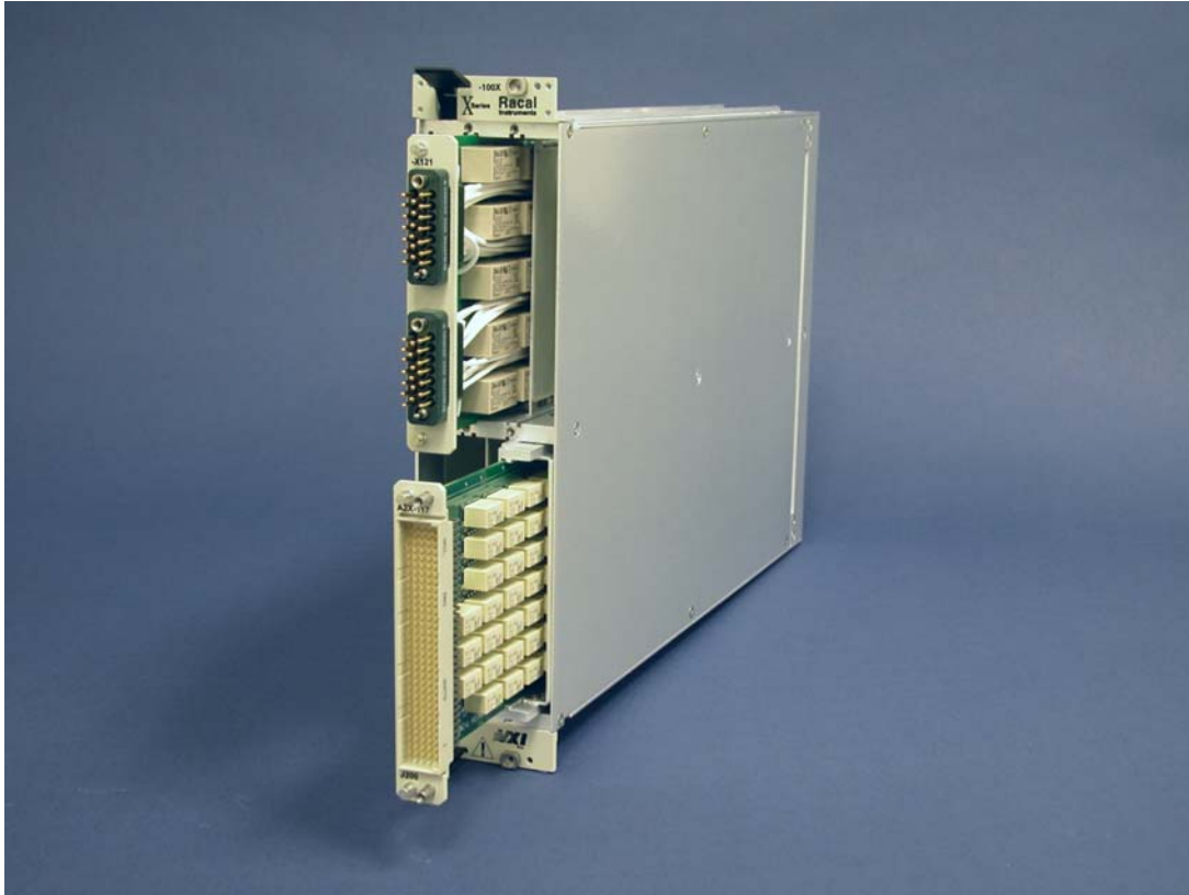
Figure 1-1, The 1260-100X Shown with Two X-series Adapt-a-Switch Cards Installed
